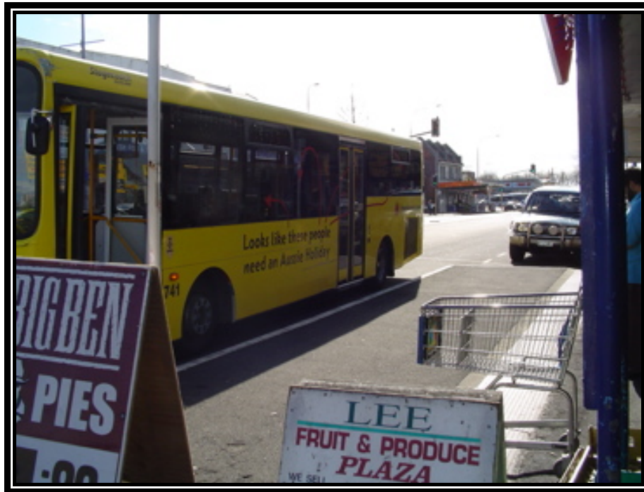
Photo 5: An example of a bus boarder, Grey Lynn. This example also highlights the need for access to a bus stop to be free of side walk clutter that would restrict wheelchair access or visually impaired or blind persons from safety accessing a bus stop. For controls on Signs refer to Council's Consolidated Bylaws.
